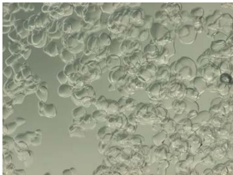
Fig. 5.14 - Slurry ice with propylene glycol as depressant
